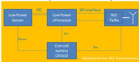
Figure 2: Schema block of Bluetooth Smart<sup>®</sup> sensor modules
