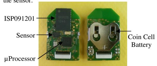
*Figure 1: Bluetooth Smart<sup>®</sup> sensor module: top and bottom views*
