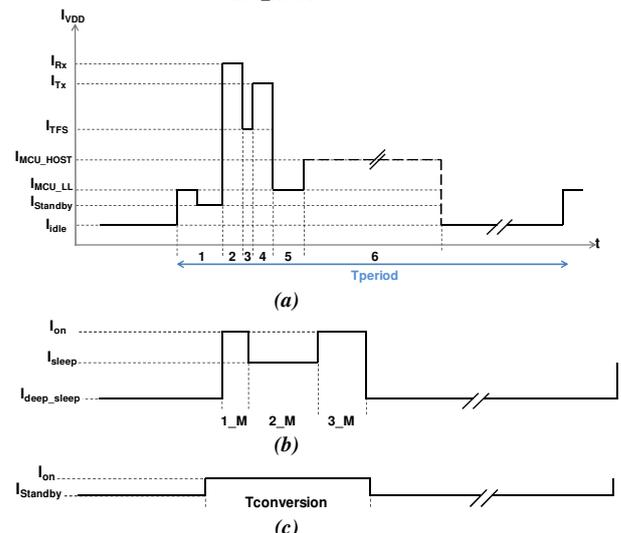
Figure 4: Current consumption over time for the module ISP091201 (a), for the microprocessor LPC1114FHI33/302 (b) and for the sensing device (c)
