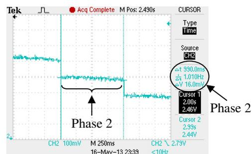
Figure 11: Temperature sensor node: total current consumption measurements during Phase 2, as measured by capacitor method
