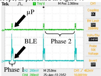
Figure 6: Two functioning phases, as measured by oscilloscope method
