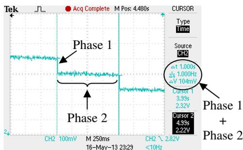
Figure 9: Temperature sensor node: total current consumption measurements, as measured by capacitor method
