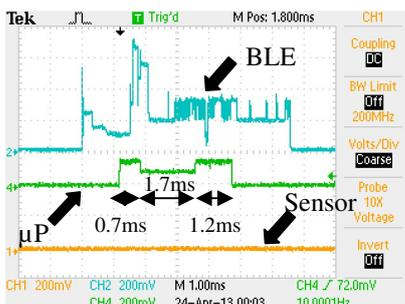
Figure 7: Temperature sensor node: current consumption measurements of BLE module, microprocessor and sensing device, as measured by oscilloscope method
