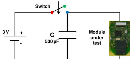
Figure 8: Electrical schematic for current consumption measurements, using capacitor measurement method
