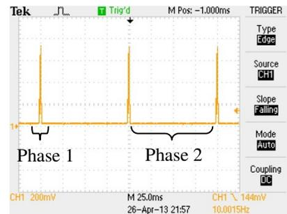
Figure 3: Operational phases of the Bluetooth Smart<sup>®</sup> sensor nodes
