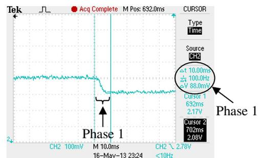
Figure 10: Temperature sensor node: total current consumption measurements during Phase 1, as measured by capacitor method
