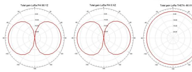
Note: The radiation pattern shape is the same in all the simulation, only the values will change with the PCB dimension.
