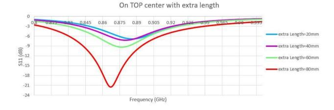
The table below represents the results of the simulation at the resonance frequency fr=868MHz, note that the length of the PCB is L=50mm and its width is fixed to 30mm.
