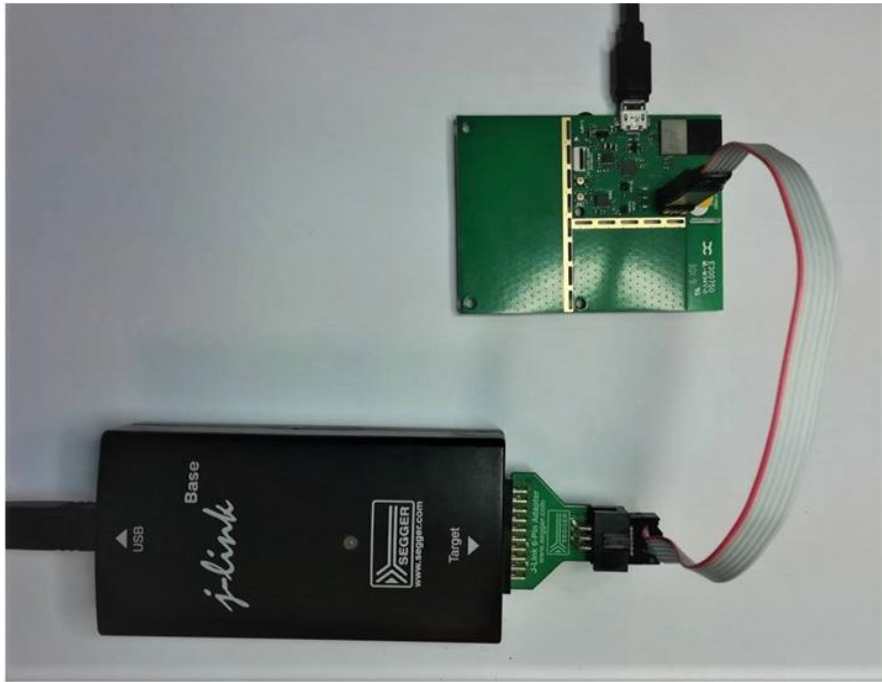
Figure 3: ISP4580 firmware loading via external JTAG
