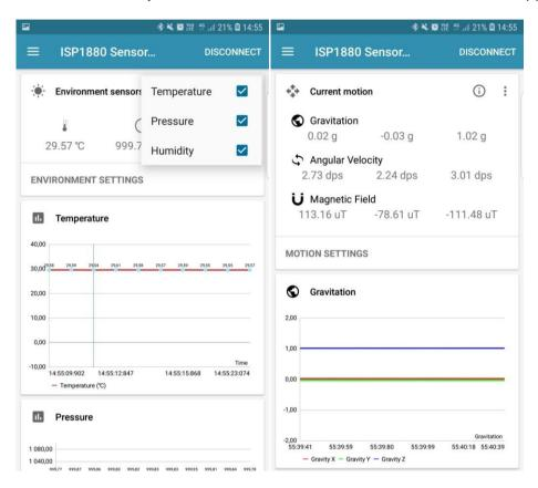
4. For the motion sensor, click on the top left part of the screen to move to the motion sensor. A calibration phase is needed to ensure a good motion. We invite you to rotate the ISP1880 Sensor Board. Then you can move the sensor on all the direction you want to see the plane moving in real time.
